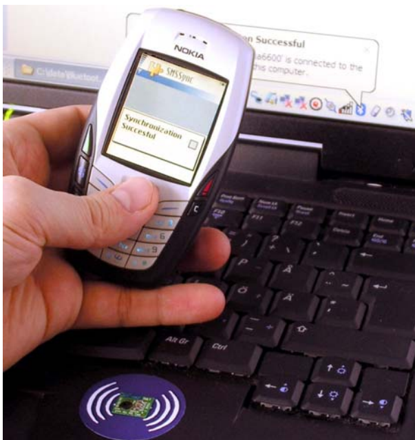
Figure 5. SMS messages are sent to the PC by touching the RFID tag.
