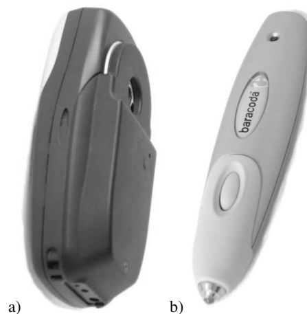
Figure 1. Nokia 6600 phone with RFID reader attached (a) and a Bluetooth barcode reader pen (b).
