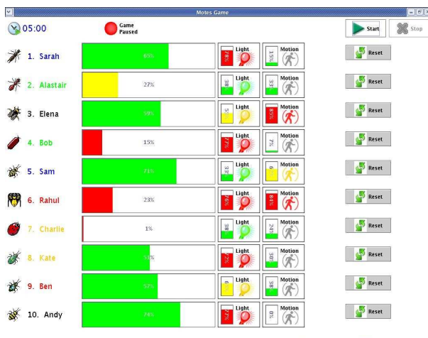
Figure 1: The graphical interface of Trove during a ten-player game. The bars next to each players name indicate the amount of lives left. On the right of each health bar are two indicators showing the current status of each players light sensor and accelerometer.
