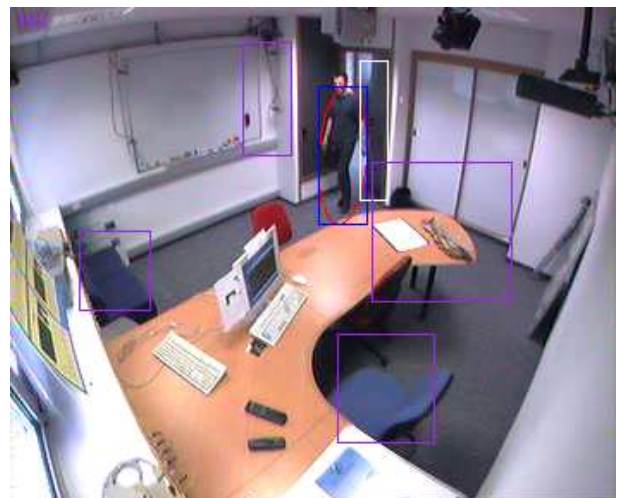
Figure 5: Video image of the wide-angle camera of SmartOffice. Four presence detection zones of the tracking system are indicated. A white box next to the door is used for the creation of new targets (entities). One person is currently tracked.
