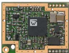
Figure 2: Wavefront OEM card with Wavenis RF transceiver
