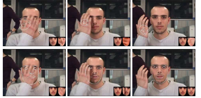
Fig. 4. Tracking on a video sequence with occlusions, frames 921, 928 and 940. Top row: deterministic AAM tracking. Bottom row: CONDENSATION based tracking.
