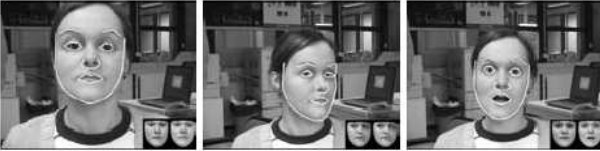
Figure 3: AAM-based adaptive CONDENSATION tracking, for frames 69, 109 and 188. On each image, the drawn shape shows the estimated state \hat{\mathbf{x}}_t ; the model and image texture \mathbf{g}_{model}(\mathbf{c}_t) and \mathbf{g}_{im}(\mathbf{p}_t, \mathbf{c}_t) are displayed in the lower right corner
